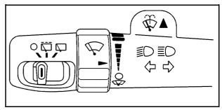
$\Psi$  : Single wipe, turn to  $\Psi$ , then release. Several wipes, hold the band on  $\Psi$  longer.
